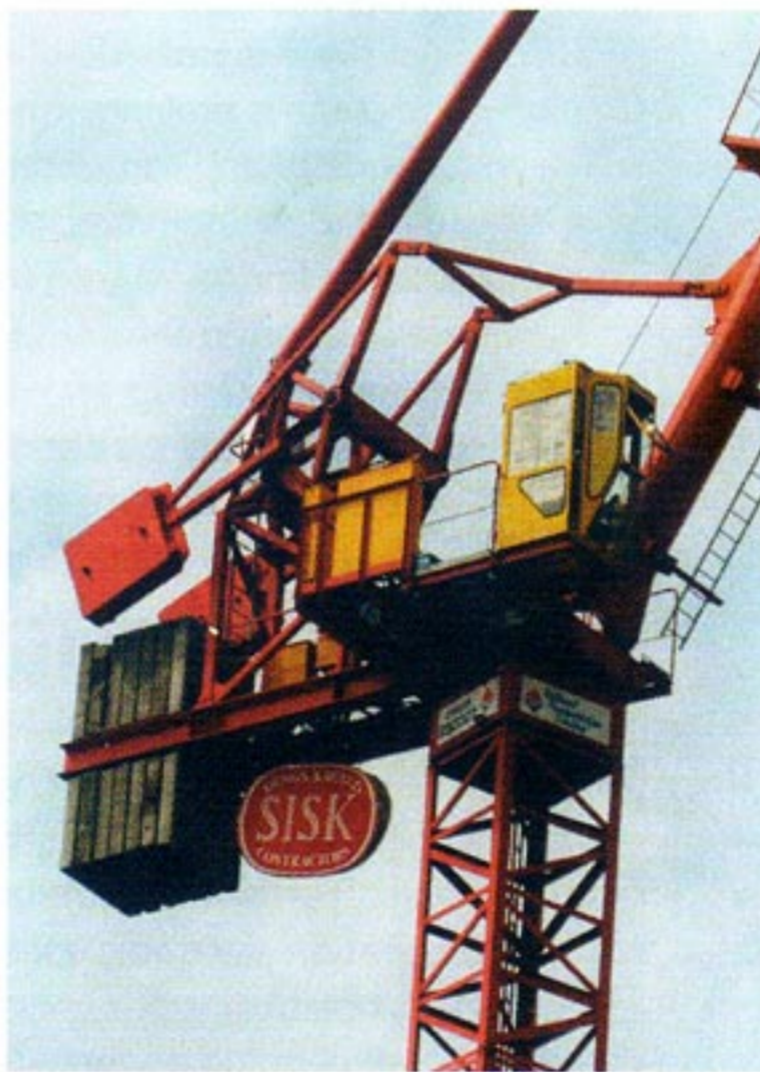
Detail of the Kroll K 103 V machinery deck showing the fixed ballast and movable steel ballast
